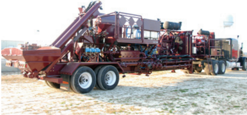
Combination Frac/Blender unit bound for West Texas
