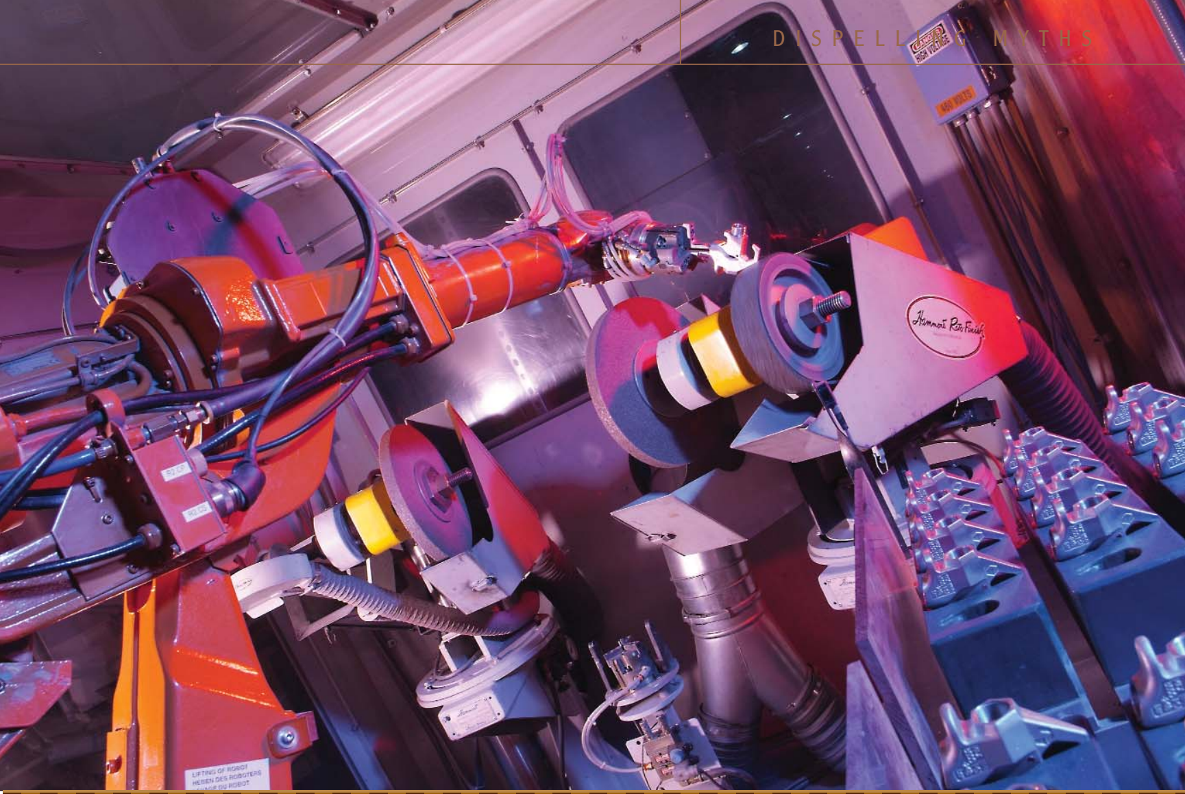
The robotic buffing cell used for Graco's Contractor™ II gun.
