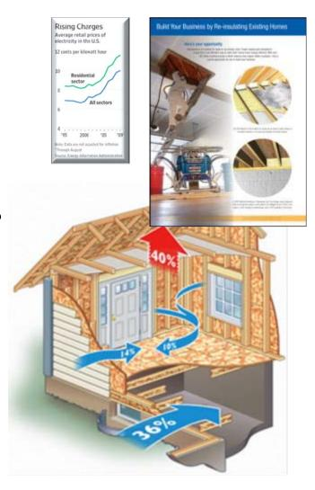
Picture shows typical air leak issues in homes and the increased energy loss
